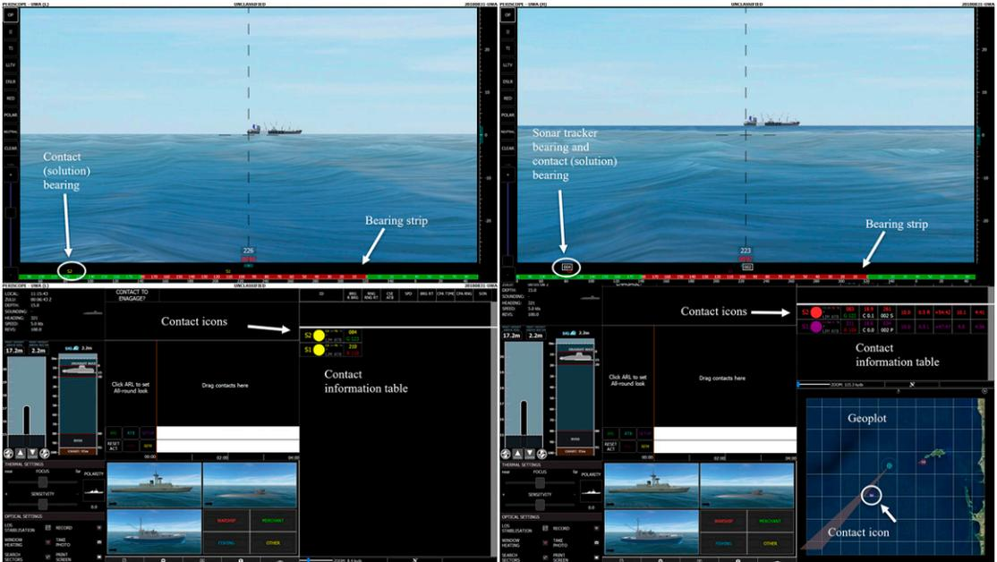
Figure 4. The Periscope display as presented to the low integration (left) and high integration (right) conditions. For high integration, the TMA solution bearings, sonar tracker bearings, contact classification (color of contact icon), the solution range, course and speed information, and Geoplot were presented. For low integration, only the contact (solution) bearings were presented. TMA = Track Motion Analyst.
