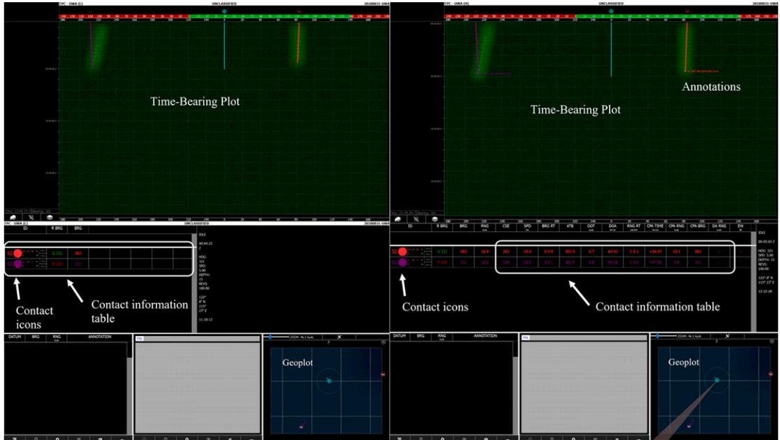
Figure 5. The Track Manager displays as presented to the low integration (left) and high integration (right) conditions. The difference between integration conditions was the presentation of additional contact information in the contact information table, such as the TMA solution range, course, speed and bearing rate in high integration but not in low integration, as well as time-bearing plot annotations from TMA and Sonar. TMA = Track Motion Analyst.
