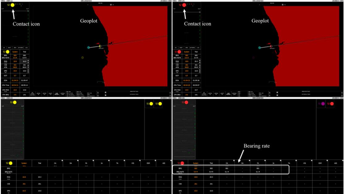
Figure 6. The Track Motion Analyst (TMA) displays as presented to the low integration (left) and high integration (right) conditions. The bearing rate and classification colors for contact icons were available in high integration but not in low integration.
