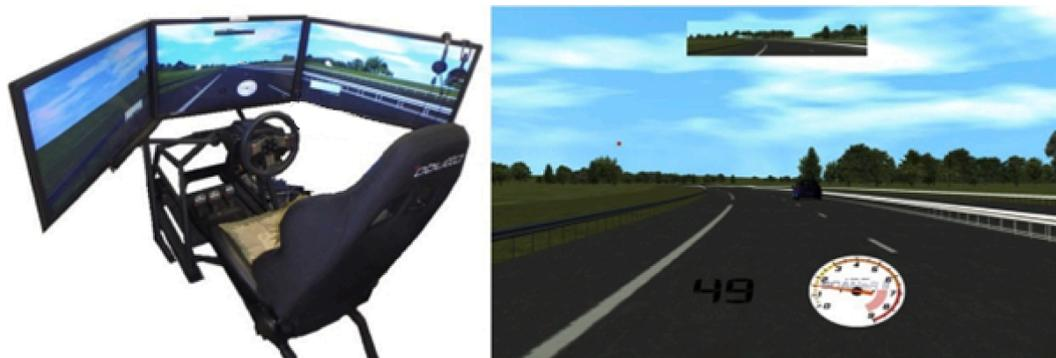
Fig. 1. Left image shows the driving simulator cockpit and displays. Right image shows central monitor with four lanes and DRT stimulus visible.
