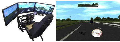
Fig. 1. The left panel shows the driving simulator with the tablet device positioned next to the steering wheel. The right panel shows the central monitor view of the driving environment with rear-view mirror and digital speedometer displayed. A DRT target is presented above the horizon on the left.
